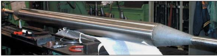
Fig. 3 — This \text{Ni}_3\text{Al} furnace roll enables increased energy efficiency, and results in higher productivity and improved product quality in the production of steel. Efficiencies result from not having to shut down austenitizing furnaces for frequent grinding to remove blister or fatigue cracks.
