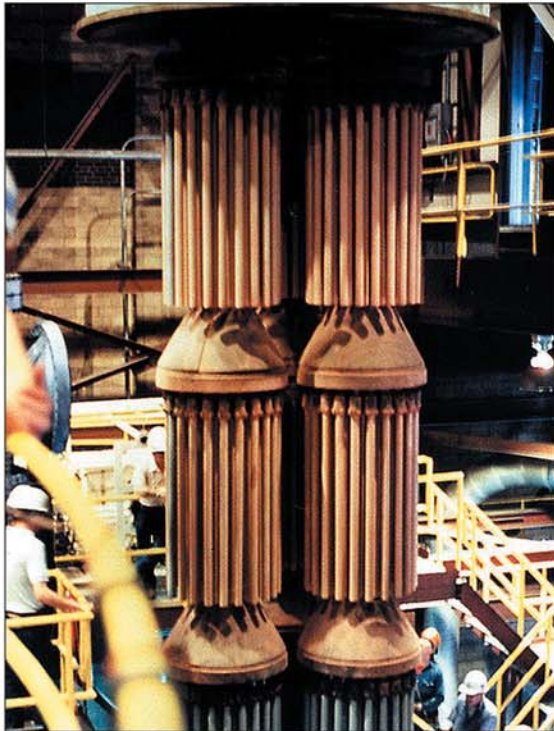
Fig. 4 — Continuous-fiber ceramic composites (CFCCs) make tough, lightweight gas filters. They function well at elevated temperatures, prevent damage downstream, reduce downtime, resist corrosion, and diminish emissions.
