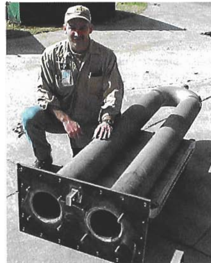
Hairpin radiant tubes made of cast nickel-aluminide tubes
