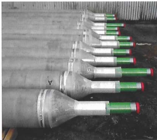
Centrifugally cast nickel-aluminide furnace rolls with trunnions welded on for use in plate mill heat treating furnace
