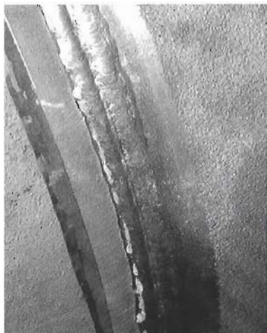
Centrifugally cast nickel-aluminide furnace rolls with trunnions welded on for use in plate mill heat treating furnace
